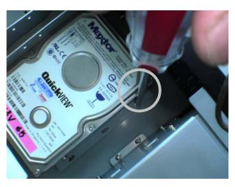
Figure 9: Attach the bracket to the DVR
